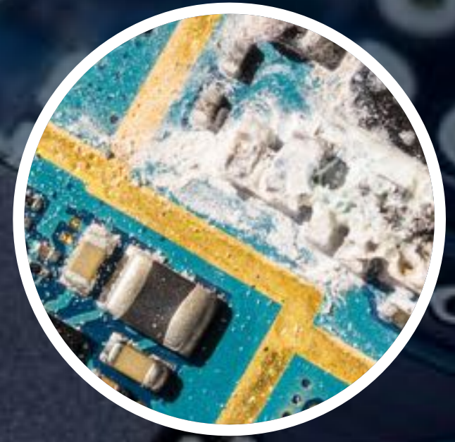
Condensation Corrosion on Cooled Components
