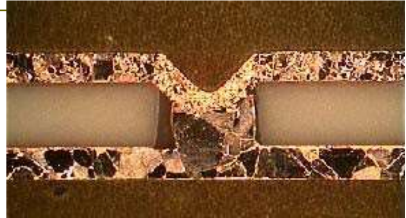
One side flat surface. Ceramic hole diameter min. 1.0mm R < 100\mu\Omega
