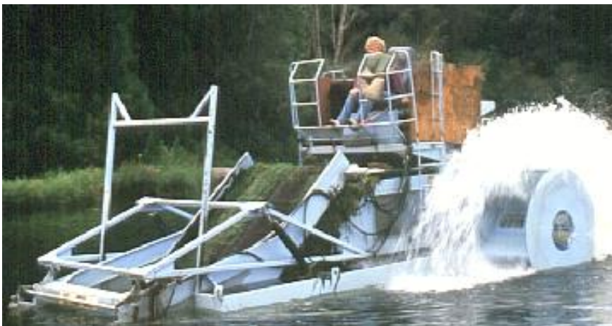
Fig. 4. Example of a harvester (from the Washington State Department of Ecology website)
