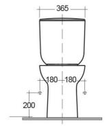
Dimensions: All dimensions in mm tollerance +5% for below 200mm and +3% for above 200mm.
