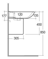
Dimensions: All dimensions in mm tolerance  $\pm 5\%$  for below 200mm and  $\pm 3\%$  for above 200mm. Note: Due to a continuing development programme to improve design and performance, the manufacturer reserves all rights to vary specifications without prior information.
