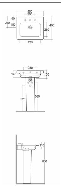
Dimensions: All dimensions in mm. Tolerance of vitreous china & fireclay items:  $\pm$  5% for below 200mm and  $\pm$  3% for above 200mm; for all other items tolerance  $\pm$  1%. Note: Due to a continuing development program to improve design and performance, the manufacturer reserves all rights to vary specifications without prior information. Please note accessories are for photographic use only.
