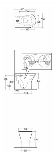
Dimensions: All dimensions in mm. Tolerance of vitreous china & fireclay items:  $\pm$  5% for below 200mm and  $\pm$  3% for above 200mm; for all other items tolerance  $\pm$  1%. Note: Due to a continuing development program to improve design and performance, the manufacturer reserves all rights to vary specifications without prior information. Please note accessories are for photographic use only.
