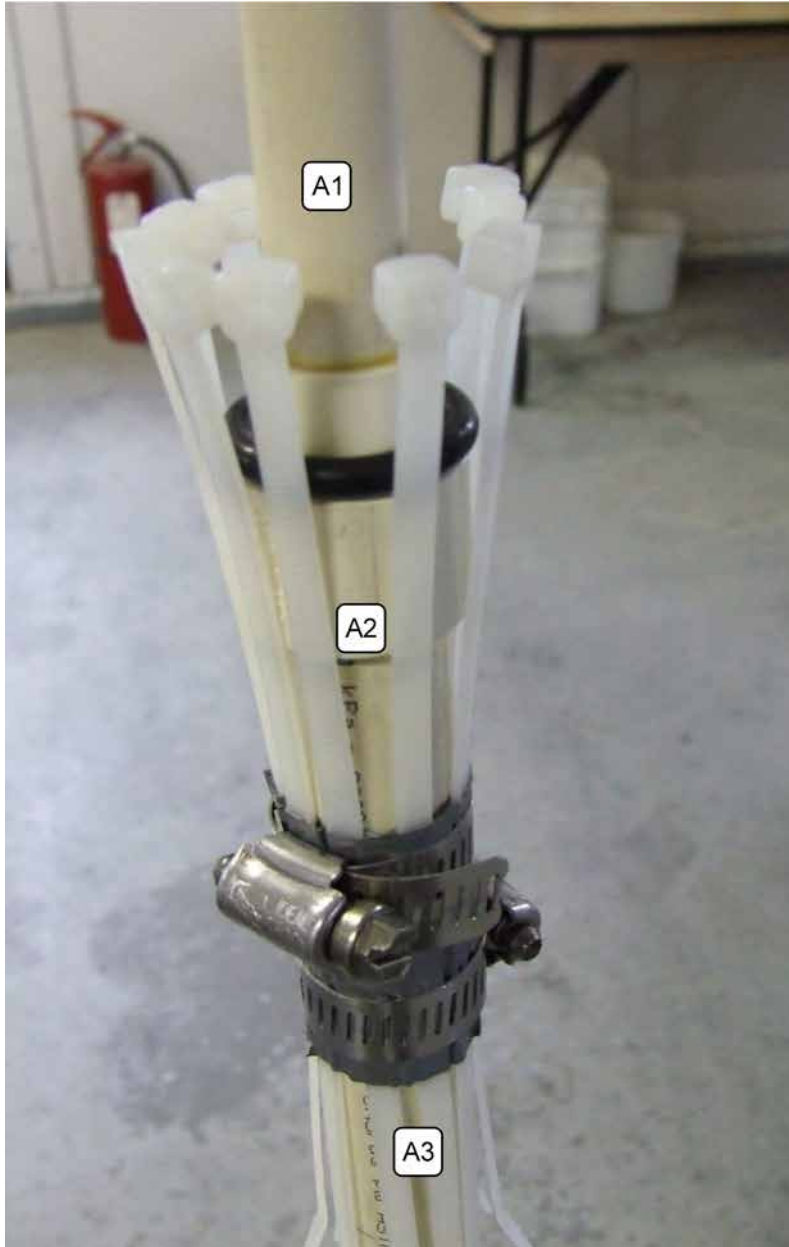
Figure 25-A Tie Cables Clamped to A3
