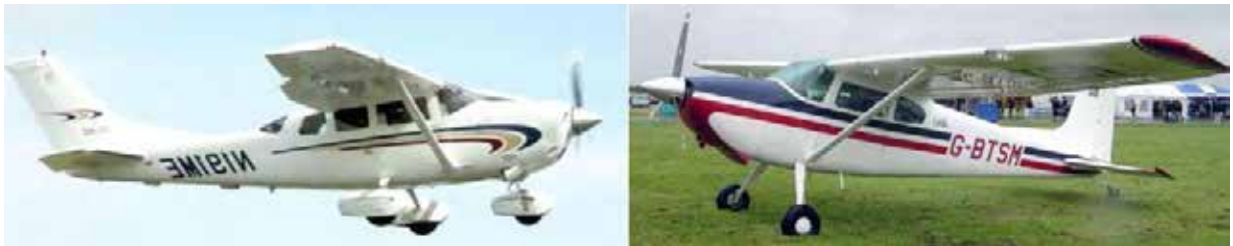
Figure 3 Nose Gear v. Tail Gear
