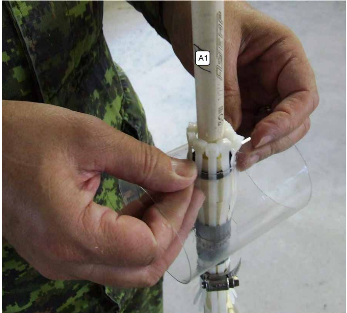
Figure 28-A Sliding the Spring over the Cable Ties
