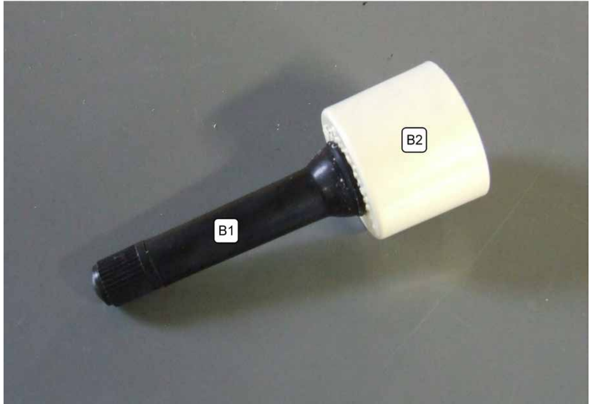
Figure 12-A Section B, Tire Valve Pulled Through B2
