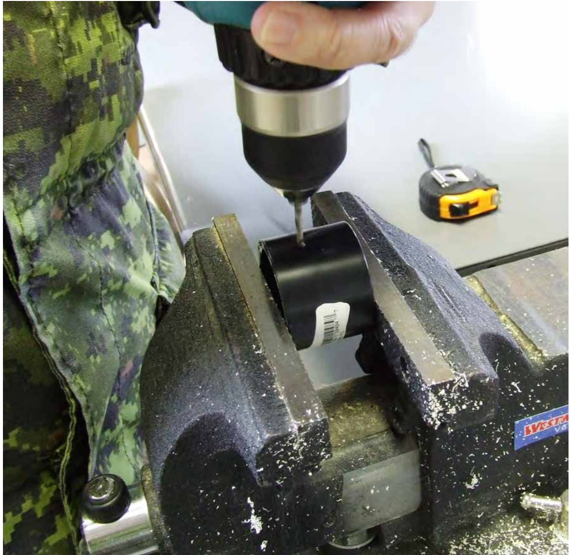
Figure 26-A Drilling 1/8-inch Holes in the ABS Coupler
