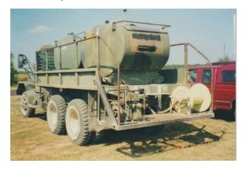
West Lake's first tender was a 5-ton deuce and a half military truck that held 800 gallons in two 400-gallon pods with a pump on the bumper.
