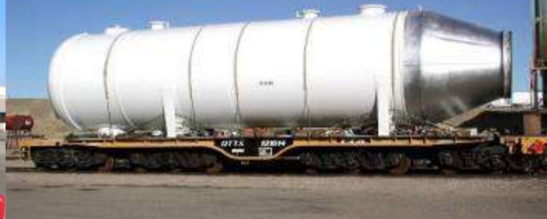
Tower, 10.5' OD, 305,000#, 200' Long, Commerce City, CO
