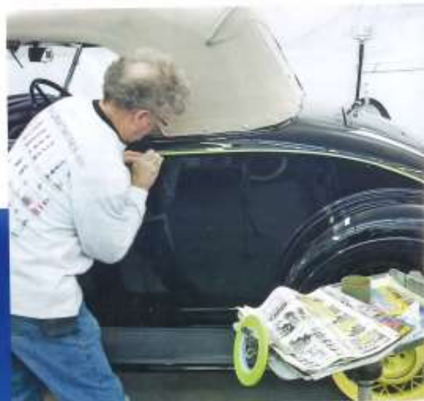
Larry Hook is beginning to pin stripe this 1935 roadster. He first runs a tape line, pulling it straight across the full length of the body. This line is used to guide his hand as he moves his brush along the body molding. Note the newspaper on the table in the foreground. He uses it as a palette to custom-mix paint to match the medium cream wheels.
