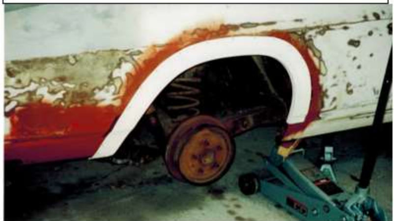
Repairing the wheel with fiberglass molding in 2001.
