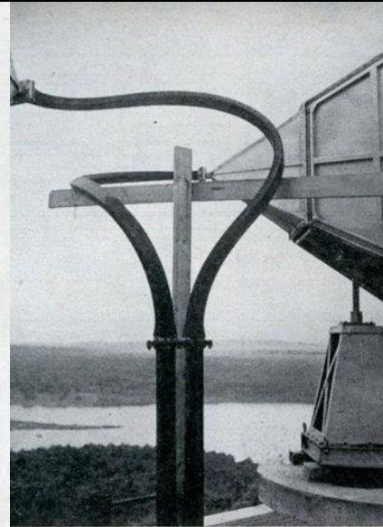
Hornlike metal lenses serve as antennas, one receiving, the other transmitting, microwaves. They focus the waves into narrow beams the way light is focused by glass lenses. The focused beams travel to and from the amplifiers below in the gracefully curving wave guides, which are hollow square copper pipes.
