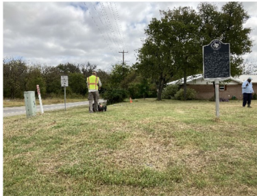
Archeologist operating a ground-penetrating radar at the Tom Cook Blacksmith Shop, where the "Bolivar" historical marker is located.
