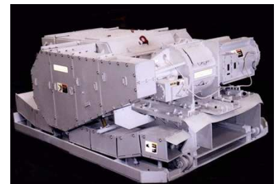
Figure 3. Coal Crusher, Belt Driven.
