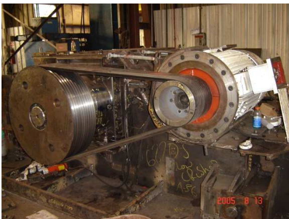
Figure 46. Motor Face Mounted to Hinged Cradle.
