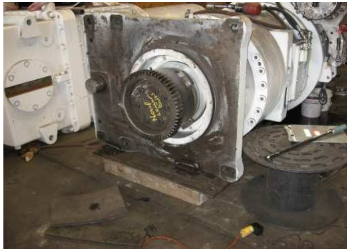
Figure 31. Two-Stage Planetary Gearbox Supported On Rubber Sheets and Wood Beams to Lower the Mounting Frequency for Balancing.
