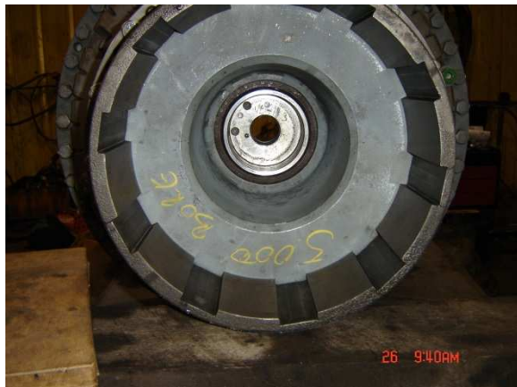
Figure 17. Voith Fluid Coupling Input Showing EPK Type Flexible Coupling Hub. Ref 4
