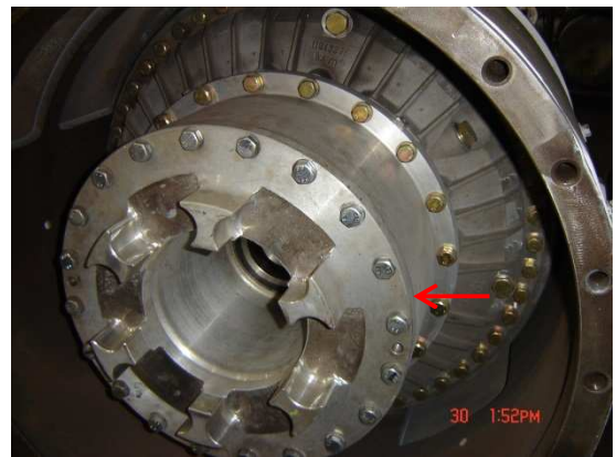
Figure 36. Modal Test Point at End Of Fluid Coupling, Input End, Horizontal Direction.
