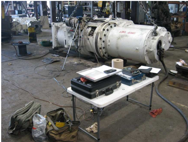
Figure 28. A Power Unit Setup to Trim Balance The Fluid Coupling In-Situ.
