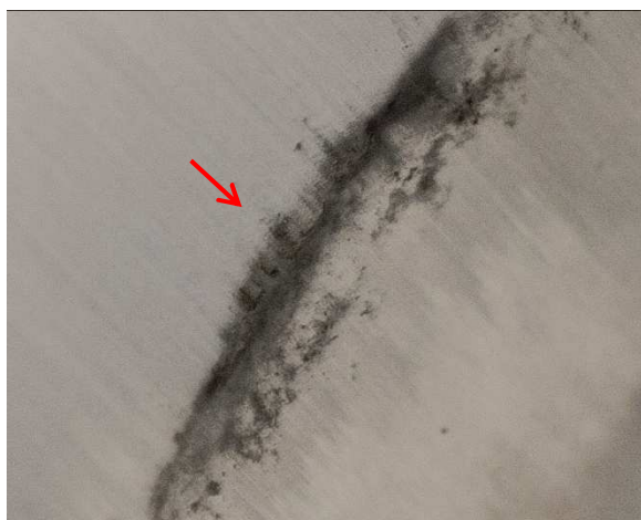
Figure 25. Motor OB Bearing Inner Race False Brinelling.
