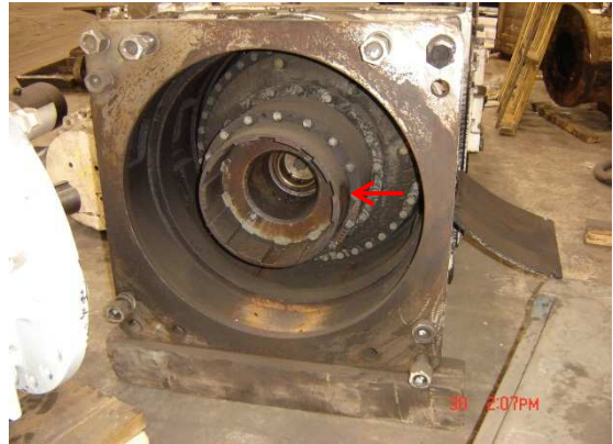
Figure 35: Modal Test Point at End Of Fluid Coupling, Input End, Horizontal Direction.
