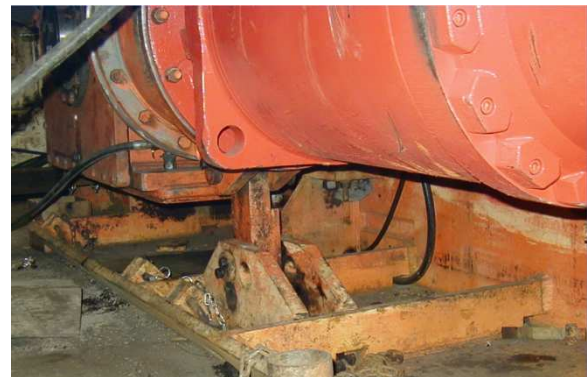
Figure 50. Link Connecting Coupling Housing to Crusher Frame to Resist Rotation Torque.
