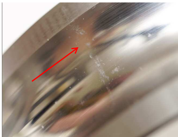
Figure 27. Motor OB Bearing, Inner Race False Brinelling.
