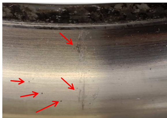
Figure 26. Motor OB Bearing, Outer Race False Brinelling and Pitting.
