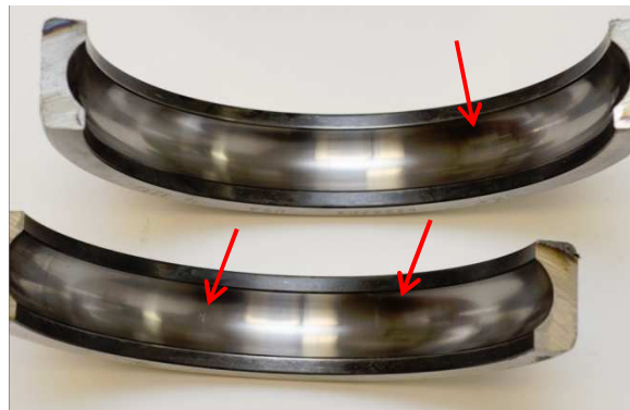
Figure 24. SKF 6224 Outer Race Showing False Brinelling Damage.
