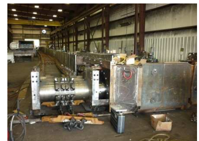
Figure 2. Conveyer Power Unit, Sprocket and Chain.
