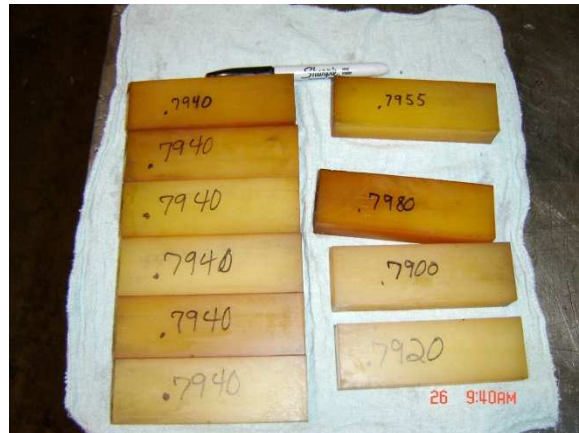
Figure 18. EPK Coupling Elastomeric Blocks Showing Measured Thickness.
