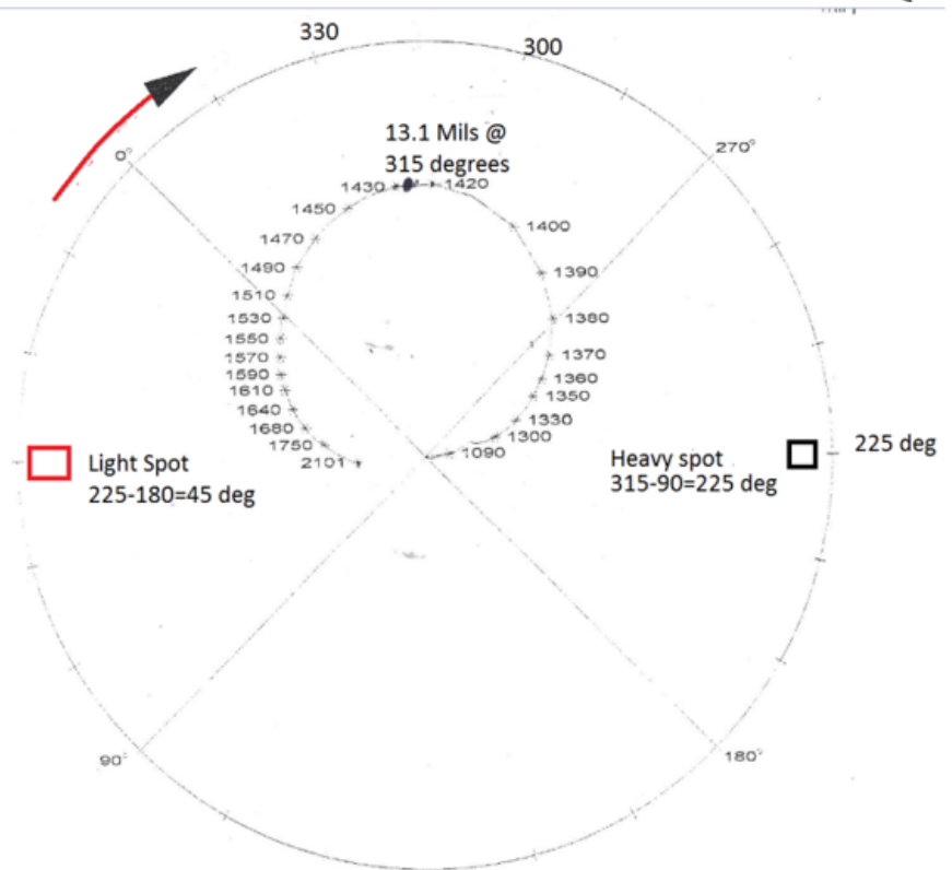
Figure 20 Nyquist plots showing 1 st critical speed response
