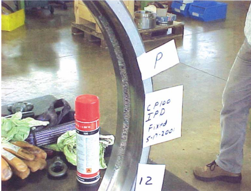
Figure 16. Advanced Spalling of Bearing Described in Figure 15. Spalling Over 45 Degree Arc of Outer Race
