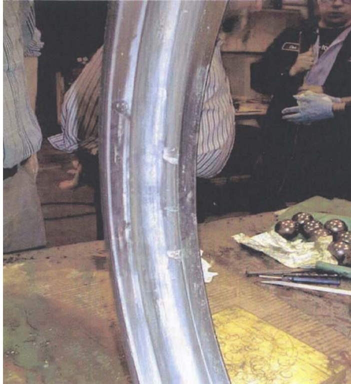
Figure 14. Beginning of Spalling of Bearing Described in Figure 13. Spalling Over 5 Degrees of Arc on Outer Race
