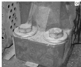
Figure 33. Bearing Housing Hold Down Bolt Washers Dished, Full Shim not Used Under Housing.
