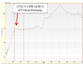
Figure 28. ID Fan A, OB Pedestal FRF Reference DOF 135X:135X.
