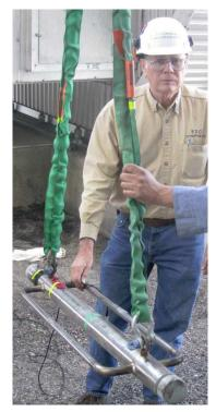
Figure 26. Author <sub>(Singleton)</sub> With Steel Ram Equipped With 50,000 lb<sub>f</sub> Force Head Supported by Nylon Slings.
