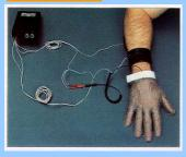
Fig. 3: MESH-Glove (MESH). 2-channel stimulation device (50 Hz, pulse width: 250  $\mu$ s). Subthreshold stimulation at 0,9-1 mA.
