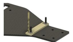
Install the 3x20mm screws into the new holes. Install a plain nut and then the post. Do not overtighten. Install a bearing, the steering arm, and another bearing for each side. Install a washer and 3mm locknut on each, again do not overtighten. Install the steering drag link to the arms with a shim on each side of the ball joint as shown. You will be relocating your steering servo 90°. Attach the linkage as needed for you fitment.
