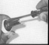
STEP 7: At this time check for smooth diff rotation. If diff is not smooth, disassemble diff backwards through the steps until you find the problem and have it corrected before continuing on. Now put drive adapter #234 or #235 into place on thrust plate and line up three holes. Install the three small 2-56 screws and tighten down with regular size screw driver. Be sure they are good and tight, because if they come loose (out), they will cause severe damage to the belt and gears.
