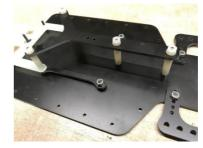
4-40 x 1/2" (4) 4-40 x 3/8" (4) 4-40 x 3/4" (3) 4-40 setscrew (4) 4-40 set screw (2) Tweak 4-40 plain nut (8) 4-40 nylon (4) 4-40 nyloc (4) Thick washer (2) 4-40 standoff 15/16 or 25mm (2) 4-40 standoff 13/16 or 20mm (2) (cut down)
