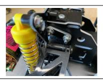
Step 15: Install the two shock tower screws.
