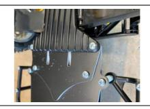
Step 17: Attach the front portion of the nerf bars to the chassis using screws and nuts. These help hold the front of the chassis together so please do not delete the nerf bars. Attach the driver figure if you wish using screws and nuts. He will sit pretty low in the body. Install your electronics.
