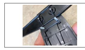
Step 6: Install the bumper onto the front chassis using nuts. Note how we have trimmed out bumper for a better and cleaner fit.
