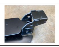
Step 10: Install the locking lower plate using 2 of the battery standoff posts and screws to hold it.
