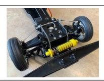
Step 9: Slot the upper and lower chassis plates and brace into the rear plates.
