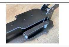
Step 12: Install the shock tower brace to the upper brace plate using short screws and nuts.
