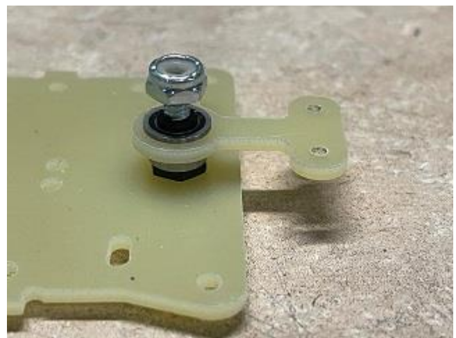
crank installed onto post. Second flange up also
