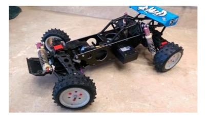
You can bolt the servo in place as original, or run the Team Associated bellcrank steering set part number 6255. We include a long 8-32 button head screw and nuts. The bellcrank is Associated part number 6281. Install as shown in the pic, upside down from a typical rc10 install. You will need to use 3mm threaded rod to make new tie rods and an additional linkage to the steering servo.
