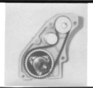
STEP 2: Put the short end of top shaft/pulley into top bearing of right case half (one without hole). Then install idler pulley & diff. Install diff going into right case half so that diff adjustments are done on the left side of tranny. Then put belt around top pulley first, loop to back of idler and slide on to diff gear as in above picture. Spinning top shaft will help bring belt down on diff gear.
