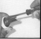
STEP 7: At this time check for smooth diff rotation. If diff is not smooth, disassemble diff backwards through the steps until you find the problem and have it corrected before continuing on. Now put drive adapter #234 or #235 into place on thrust plate and line up three holes. Install the three small 2-56 screws and tighten down with regular size screw driver. Be sure they are good and tight, because if they come loose (out), they will cause severe damage to the belt and gears.
