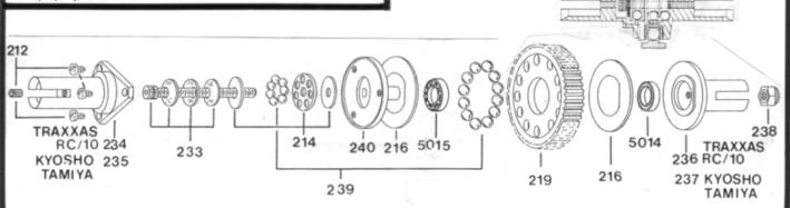
RC/10 & RC/10T It is recommended that you drill two new mounting holes in chassis for front of tranny. For proper hole locations, a drill jig #227 has been supplied to you with your new Lethal Weapon 2. To do this you will need to remove rear bulkhead, stock tranny and suspension from chassis.
