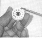
STEP 2: Keeping the diff ring locked in place, put the diff gear onto the thrust plate. Using a small screwdriver put some of the light grease in each of the holes of gear. Once their all packed, place a 1/8" ball into each hole (larger ones). Set assembly aside for now.
