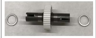
Reassemble your Stealth differential using the supplied Factory Works diff balls, diff gear, and special adapter bearing. Make sure that the T-nut and spring are installed into the male outdrive. We recommend using Stealth diff lube and black grease. If you require step by step instructions, they can be found on the Team Associated website.
