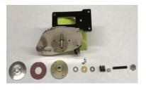
Install the 6/32 set screw into the topshaft with loctite. Hold the shaft with the pin in the hole of and tighten until it stops against the pin. Slide the inner slipper hub onto the shaft and onto the pin. Press the supplied bearing into outer slipper hub. Center the clutch disc onto the outer slipper hub and carefully slide the assembly onto the shaft.
