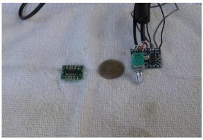
the picture the one hooked up comes with the volume control and off/on switch on the board and cost about \$4.00. The other without the volume and power switch is under \$2.00. I hooked mine up to 2 surplus speakers and it sounds not only good, but also has a great volume level. On Ebay do a search for PAM 8403 to see amplifiers for sale.
