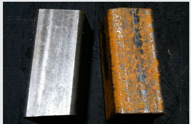
With Protection Without Protection Humidity and Salt-Spray Testing ASTM D-1748
