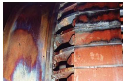
Rotor core damage due to broken bars
