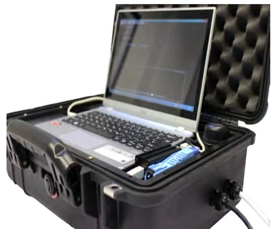
remote access using mobile broadband modems connected to the netbook computer of the data logger kit (provided there is mobile broadband coverage).
