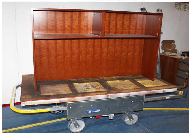
(Right) - Correct Balanced Loading
