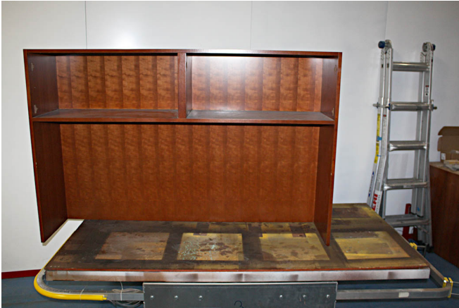
(Left) - Incorrect, Unbalanced Loading
