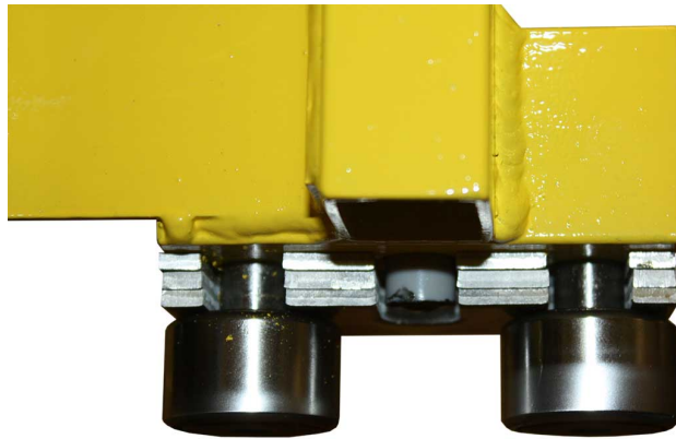
Track Sensor Reverse view, notice it's flush with the spacers
