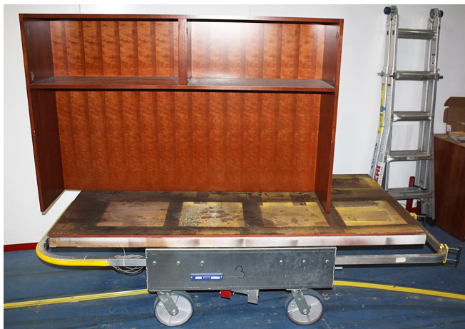
(Left) - Incorrect Unbalanced Loading
