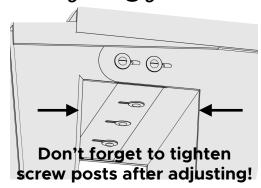
Using handle slot as guide with box on bike, drill two holes
