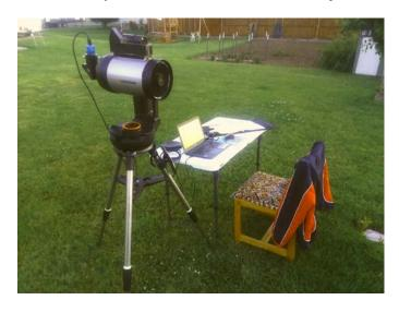
The equipment shown includes a Mallincam SkyRaider DS287/c camera with a 0.5x focal reducer screwed onto the 1 ½" tube on the end of the camera, and a Meade F/6.3 focal reducer screwed onto the rear cell of my 6 inch Evolution Celestron Scope. This set up gives a nice wide field of view.
