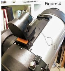
Figure 5 shows how the Polemaster is attached to my Meade 12 inch scope on the metal dovetail.
