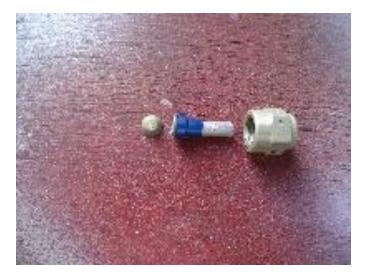
B-Nut has an un-drilled Restrictor inside
