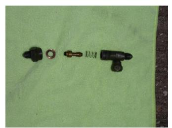
**Drilled and Undrilled Restrictors**
