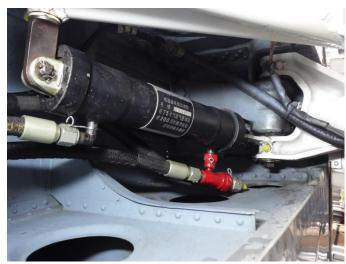
Main Gear Actuator (diverter valve in Red)
