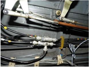
Flap Diverter Valves in Aft Cockpit
