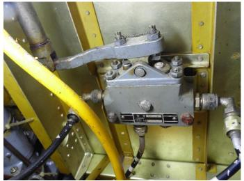
**QS-2 Brake Differential Valve** Shaft on left connects to rear rudder bar. Valve Positions are Right, Left or Both.
