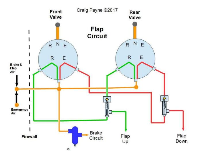
Looking at the Flap circuit, the Rear Valve must be in the Neutral position to allow the Front Valve to function. I safety-wire mine to Neutral but then keep wire cutters in the "ration box" so a *Qualified* back seater could use them in an emergency.
