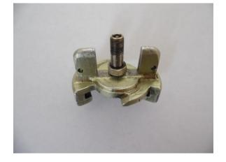
The center of the tab was milled and a 1/8" high-pressure Schrader valve was inserted into the tapped hole. The Schrader will work with or without the actual valve. Without the valve, pressure is contained by the External Fill Check Valve on the firewall. Leaving in the needle valve limits the amount of loss when the fill hose is removed.
