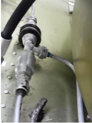
Right (starboard) Firewall Check Valves (2)
