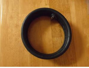
**Brake Bladder** – Heavy rubber pushes against thin metal clips and the brake blocks.
