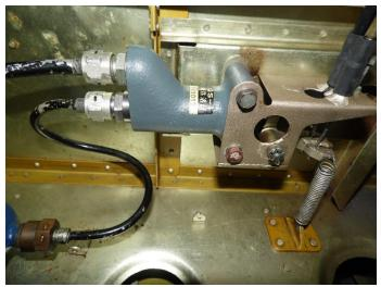
**QS-1 Pressure Reducer** Doug Sapp has seal replacement kits for servicing
