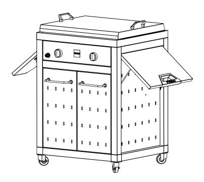
Remove the laser film from the lid. Clean the entire exterior grill surfaces with a stainless steel cleaner and non-abrasive towel. Do NOT clean the cooking surface with stainless steel cleaner. Please see griddle seasoning instructions.
