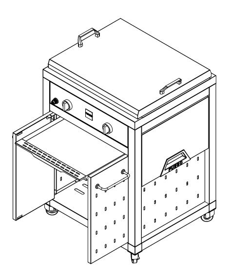
Side shelf operation. The grill can be used with the side shelves in either the open or closed position.
