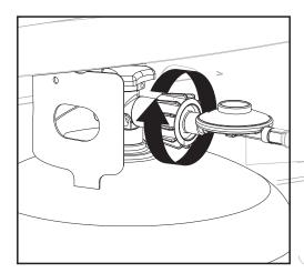
The Element by Fuego grill is orificed for use with LP gas and comes equipped with a high capacity hose and regulator assembly for connection to a standard 20lb. LP cylinder (Type 1). The LP tank is not included. LP hose and fittings are included. Operating pressure: 11" W.C.
