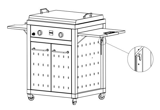
8B. To close, lift up on the shelf support brackets to allow the shelf to fold back down into the side panel.
