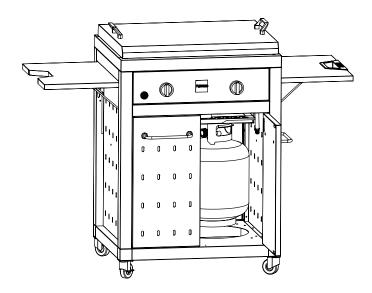
B. Connect the regulator to the propane tank. Proper procedures for gas leakage testing must be obeyed. Please note the Gas Hook-Up, Danger, and Warnings pages for more information.
