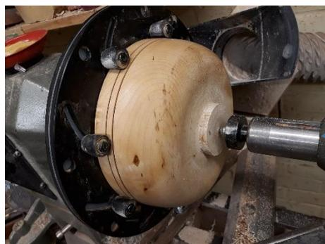
Cole jaws and Longworth style are not as secure as other jaws – keep tailstock up as long as possible and keep all force directed towards the head stock
