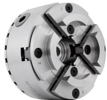
Chucks like this can hold small square stock directly, not with the jaws but inside the body of the chuck. The chucks screw directly onto the spindle of the lathe. They have a large mass and together with the mass of the blank and this means that when you turn off the lathe and try to stop it turning manually, the
