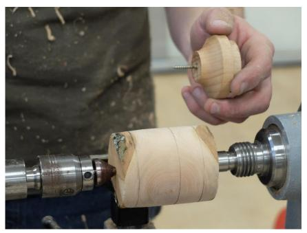
Before the final shaping the blank is removed a special screwchuck is used to mount it as can be seen in the photo.
