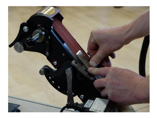
Harvey demonstrated the sharpening of a number of different gouges. He emphasised the importance of regular sharpening in woodturning and the need for controlled, repeatable and effective method for sharpening, linishing or polishing on all your edge tools. One key advantage over the grinding wheel sharpeners is that you achieve a flat edge rather than one which adopts the curvature of the wheel.
