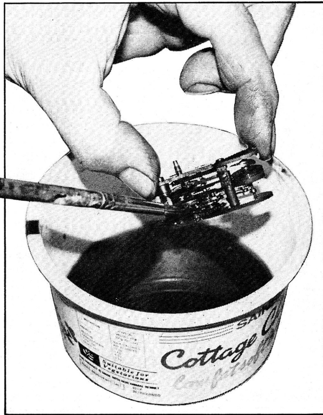
Screw and plate retain the main drive spindle. Note the particles of metal around this one; an outward sign of mechanical malaise.
