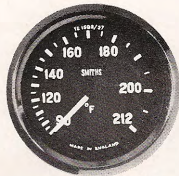
Part No. TG1502/27 Capillary Type 7' or 10' long 90°-212°F. Black Dial
