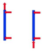
Figure 8.2 Support and restraint of curtain walling
