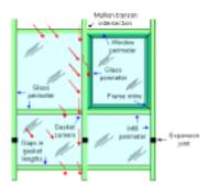
Figure 2.2 Potential leakage sites
