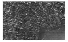
Figure 7.1 Fractured toughened glass
