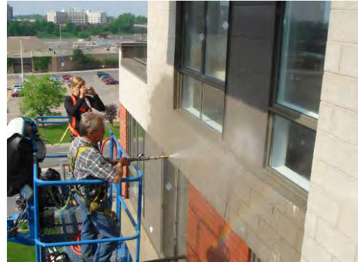
Figure 36: Diagnostic hose testing window/wall interface.
