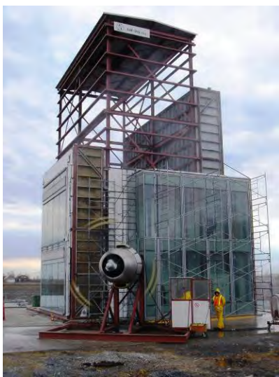
Figure 9: Exterior mock-up test (AAMA 501) - Air-Ins laboratory.
