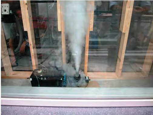
Figure 28: Portable smoke generator used to fill test chamber with white smoke.
