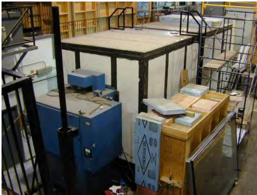
Figure 11: Environmental test chamber - Air-Ins laboratory.
