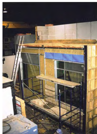
Figure 10: Interior mock-up test (CAN/CSA-A440) - Air-Ins laboratory.
