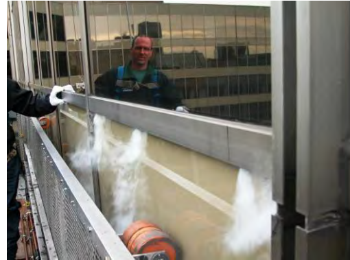
Figure 29: Excessive smoke exfiltration visible on exterior side of curtain wall test specimen.
