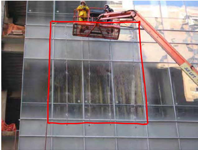
Figure 17: Identification of representative area for field testing (metal and glass curtain wall).
