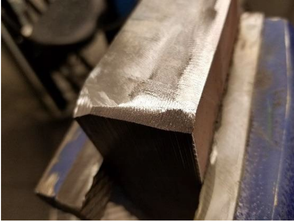
Post-grinding surface with edge removal
