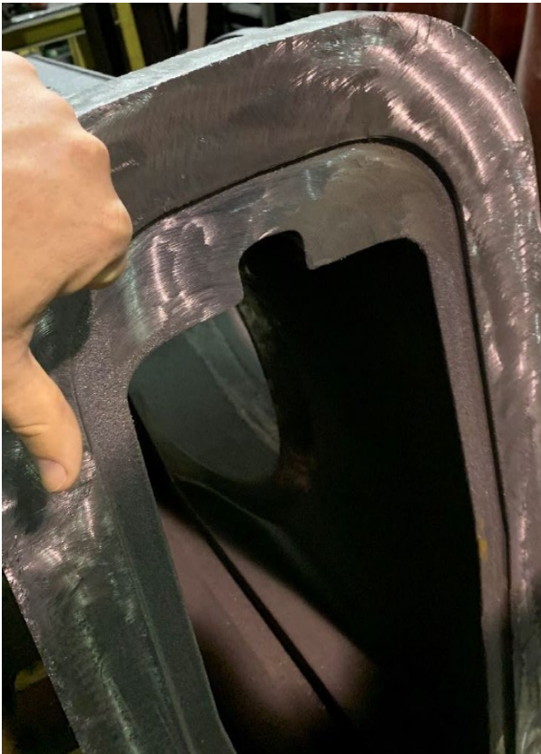
Critical gasket surface, close-up
