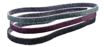
Without compromise between edge durability and flexibility, S-Flex Surface Conditioning Belts withstand critical Aerospace and General Fabrication applications requiring narrow belt operations. The semi-friable, aluminum oxide grains provide sharp cuts and consistent finishing throughout belt life and resist shedding or chunking due to their micro-fracture properties.
