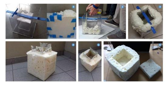
Figure 5.18: Moulding method with a mould in PVC and PU in spray  $% \mathcal{A}$
