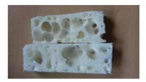
Figure 5.19: Internal structure of the PU in spray
