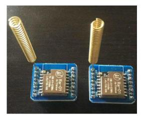
Figure 5.9: The LoRa modules
