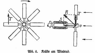
Fig. 6. Forces on the wind turbine.
