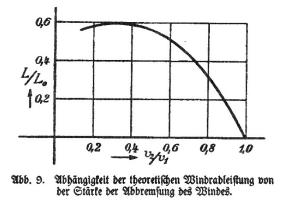
Fig. 9. Dependence of the theoretical wind turbine output on the strength of the deceleration of the wind.
