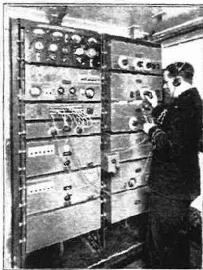
The telephone service to ships at sea was extended during the past year. The photograph shows the Marconi telephony receiver on the White Star liner Homeric.
