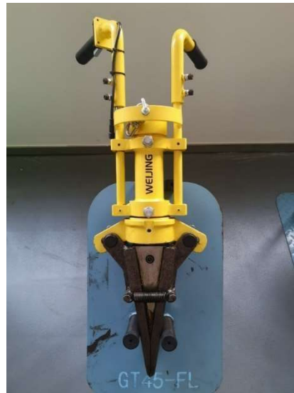
Vertical wedge for ground level degating
